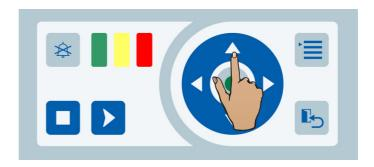
➤ The **Up** (▲) or **Down** (▼) navigation keys can be used to move to the next line up or down.
