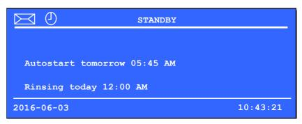
This screen shows information on the automatic rinse procedure, on the next automatic start of the system and on the next automatic heat disinfection (provided these functions have been activated).
