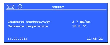
The conductivity and the temperature displayed in **SUPPLY** mode refer to the permeate outlet of the **AquaBplus B2**. The parameters of the **AquaBplus** can be viewed in the **Status - Operating data** menu.
