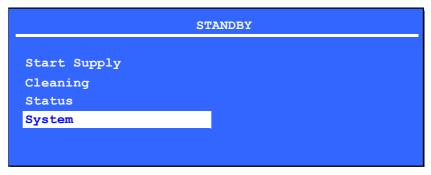
➤ When selecting the menu option **System** and confirming the selection with the **Enter** key, the System menu will be opened.
