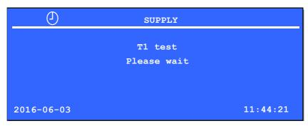
During the **T1 test**, safety-relevant components will be checked for correct function. Depending on the capacity and features of the **AquaBplus**, the test will take between 1 and 3 minutes.
