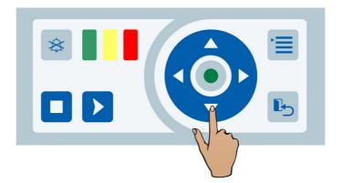
➤ The **Down** (**V**) navigation key can be used to scroll through the existing pages.
