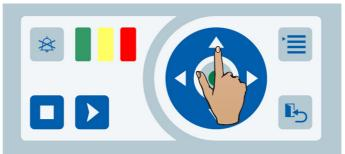
➤ The Up (▲) or Down (▼) navigation keys can be used to switch between activated / deactivated.
