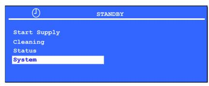
First confirm the menu option System with the **Enter** key. The **System** menu will be displayed:
