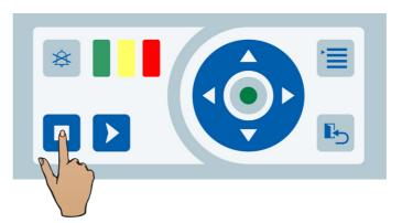
> Press and hold the **Stop** key for **two seconds**.
