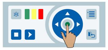
➤ Use the **Navigation** keys to select the option **Start Supply** and press the **Enter** key for **two seconds**.
