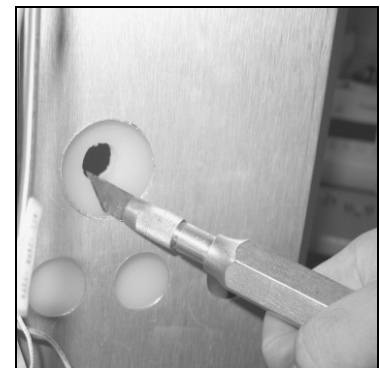
Figure 2 - New Mounting Holes
