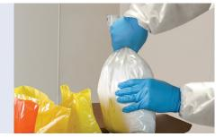
Grab the flap on the bottom of the bag and invert the bag. Insert the gathered end into the small opening in the Dry Acid Dissolution Unit.
