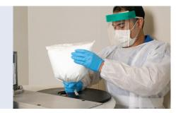
Release the gathered end of the bag and allow the contents to empty into the tank. Once all of the powder has transferred to the dissolution unit remove and discard the empty bag.
