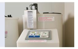
Replace the small access lid and press the DISSOLUTION START button. The Dissolution Unit will proceed to the Mix Operation. Follow the Dry Acid Dissolution Unit Operator's Manual for instructions to complete the mixing process.
