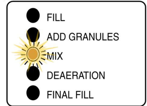
For the **GranuFlo® II Dissolution Unit**, during the **MIX** operation, the solution is mixed for a period of thirty-five **(35) minutes** allowing the granules to completely dissolve. The GranuFlo® Dissolution Unit will then automatically step to the DEAERATION Operation.
