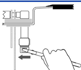
D. Remove the nut below the Spray Ball to access the Sprayer.
