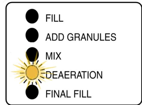
For the **GranuFlo® II Dissolution Unit**, the **DEAERATION** operation runs for **two (2) minutes** during which the entrapped air is allowed to separate out of the solution. Upon completion, the GranuFlo® Dissolution Unit will automatically step to FINAL FILL operation and the Final Fill Indicator Light will illuminate.
