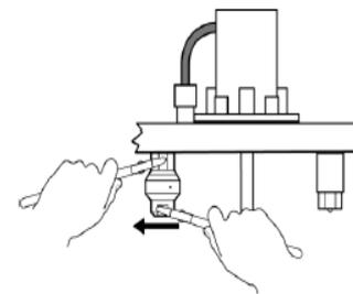
D. Remove the nut below the Spray Ball to access the sprayer.
