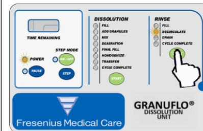
F. Press the START button on the RINSE cycle side. PAUSE light will turn off and RECIRCULATE light will not flash. Check for proper Spray Ball Rotation before continuing to pg. 10.
