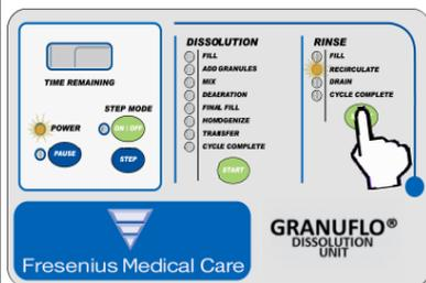
F. Turn main Power Switch ON. Press RINSE CYCLE START button. PAUSE LED will turn off and RECIRCULATE LED will not flash. Check for proper Spray Ring rotation before continuing to pg. 10.
