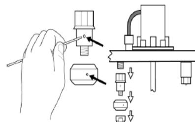
E. Clear the spray holes in both the Spray Ball and sprayer of debris and reassemble.
