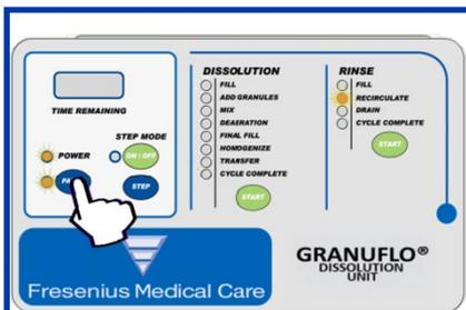
C. If the Spray Ball is stationary, push the PAUSE button. RECIRCULATE LED will flash. Turn Main Power Switch OFF.
