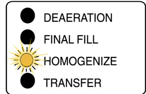
10. During **HOMOGENIZE** operation, the mixer motor will stir the solution for ten (10) minutes. When the HOMOGENIZE Operation is complete, the Transfer Indicator Light will flash. Remove Large Access Lid and look into the tank to make sure the granules have dissolved and the solution is colorless. Once you have verified the granules are dissolved and colorless, **the solution is ready for Specific Gravity Testing**.
