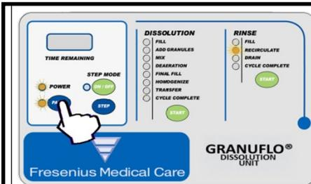
C. If the Spray Ball is stationary, push the PAUSE button. RECIRCULATE light will flash.
