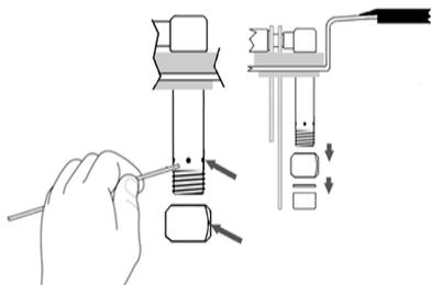
E. Clear the spray holes in both the Spray Ball Ring and Sprayer of debris and reassemble.
