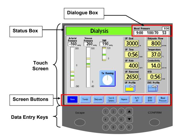
**Figure 6 – Control Panel – Treatment Display Section**
