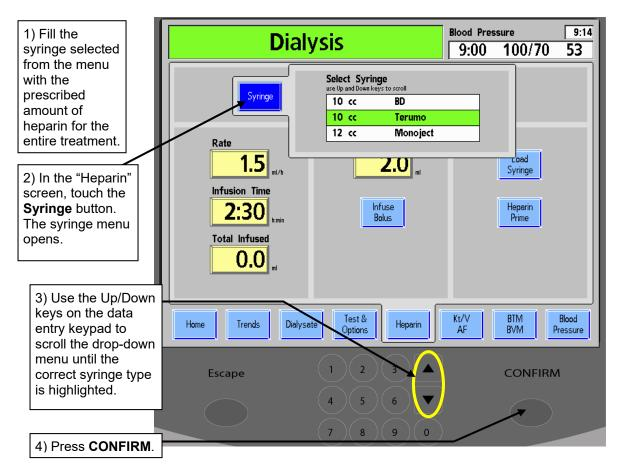
Figure 41 – The Syringe Subscreen on the Heparin Delivery Screen
