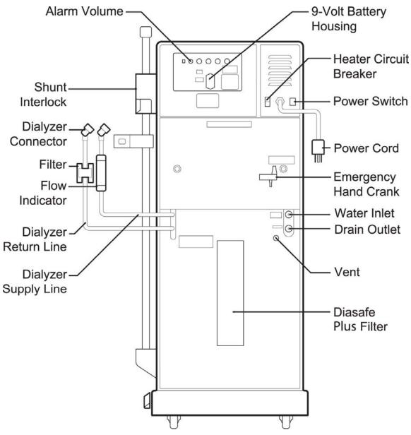
Figure 2 – 2008K Hemodialysis Machine—Rear View
