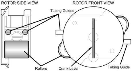
**Figure 57 – The Blood Pump Rotor**
