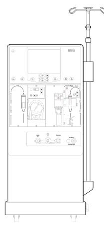
The 2008K@home hemodialysis machine is the 'home' version of this 2008K hemodialysis machine. The 2008K@home hemodialysis machine is designed especially for home hemodialysis patients. It features a shorter cabinet height, a simplified control panel, and on-screen guided treatment instructions for easier operation.
