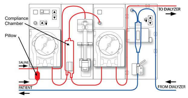
Figure 66 – Module Configuration with Digital Single Needle Pump (third module from left)
