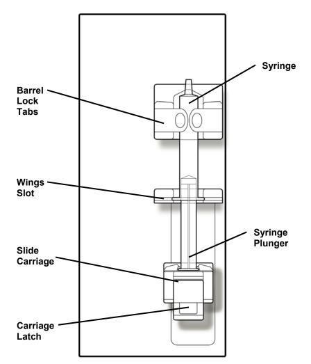
Figure 11 – The Heparin Pump Module (shown with syringe)
