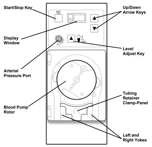
Figure 10 – The Blood Pump Module
