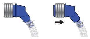
Figure 15 – Removing Dialyzer Quick-Connectors
