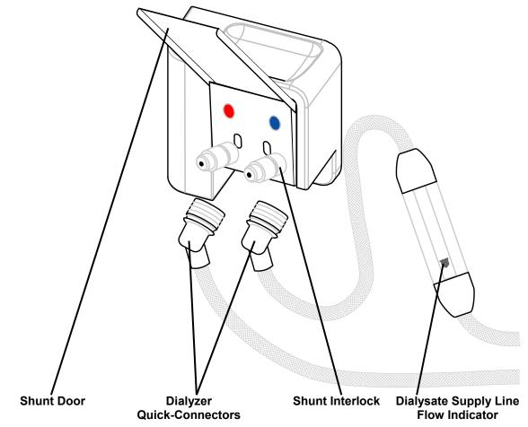
Figure 14 – Shunt Interlock, Flow Indicator & Dialyzer Connectors
