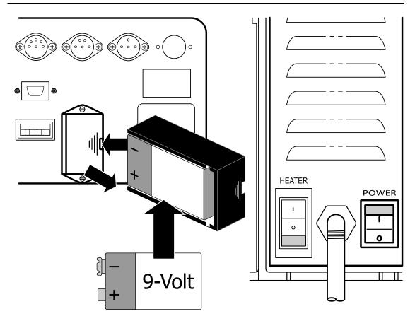
Figure 65 – Replacing the 9-Volt Battery
