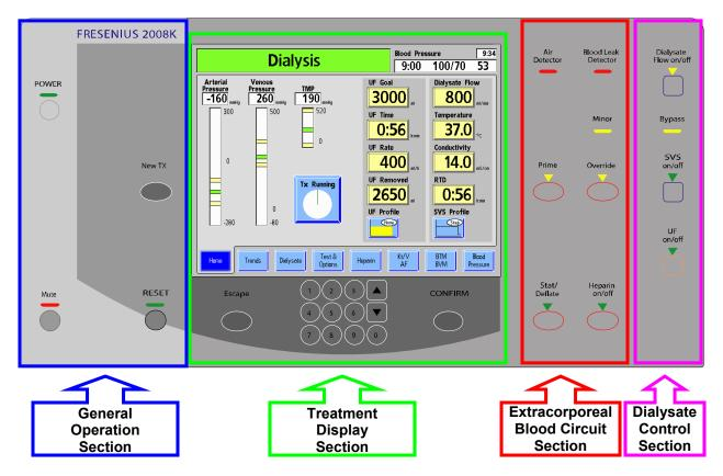
Figure 3 – The Components of the Control Panel
