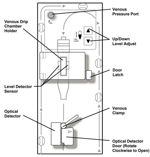
Figure 12 – The Level Detector Module
