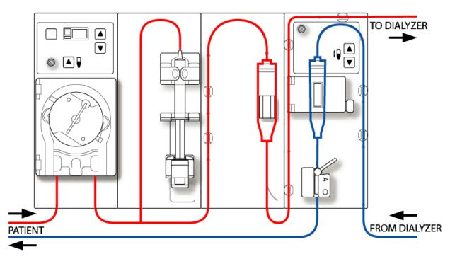
Figure 22 – Post-pump Arterial Chamber Configuration
