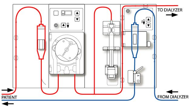
Figure 21 – Pre-pump Arterial Chamber Configuration
